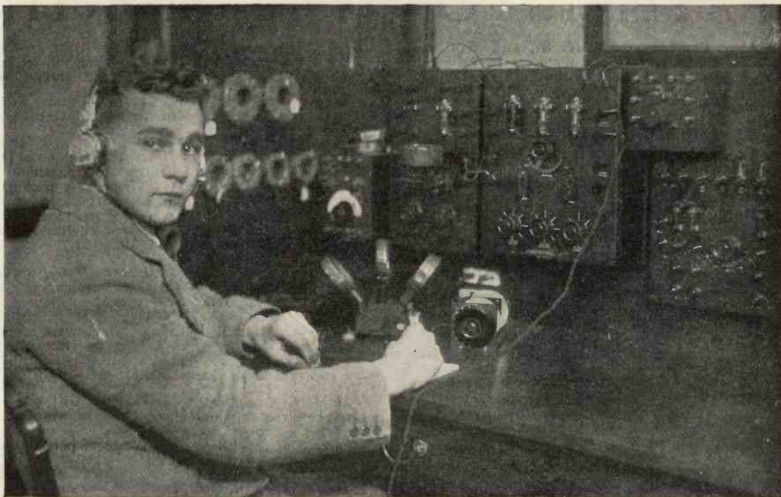
The above photograph specially taken for "Modern Wireless," shows the actual apparatus used by J. H. D. Ridley in the reception of WJZ, the Newark broadcasting station. Only two stages of radio frequency amplification were employed.
