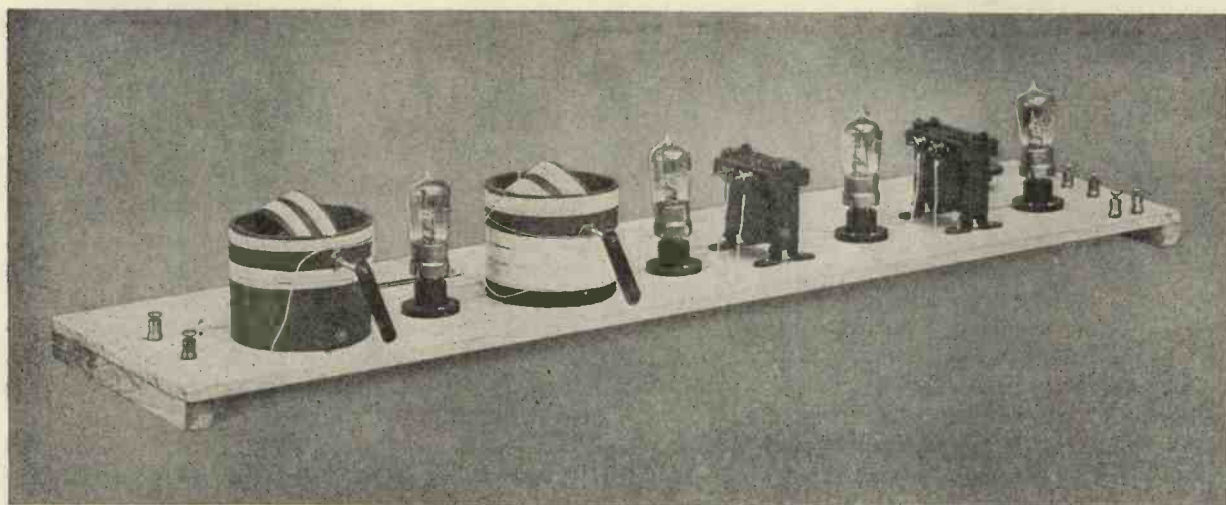
The photograph illustrates the receiver with two extra amplifying valves.
